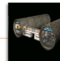
SYDNEY WESTERN HARBOUR TUNNEL 2 Slurry TBMS, 16.5 M, 6,5 km (13 km)
