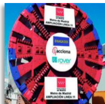
UTE L11 Metro de Madrid (SPAIN) TBM to be defined 1 EPB, 9.4 M (7.0 km)
