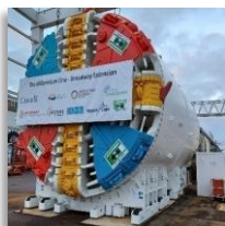
METRO BROADWAY VA. - CANADA HERRENKNECHT S-1304 HERRENKNECHT S-1305 2 EPB, 7.0 M, 5 km (10.0 km)
