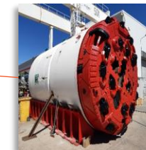
TUNEL DE MULARROYA (SPAIN) HERRENKNECHT M-949M 1 DOUBLE SHIELD, 3.5 M (13.0 KM)
