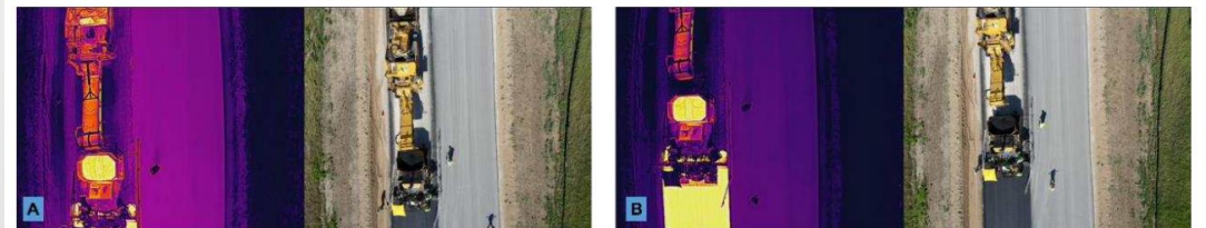
Figure 9. Thermal profile of HMA in the hopper (A) and behind the paver (B).
