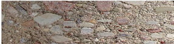
Chudy beton, f_c = 6 - 9 MPa, 20cm
