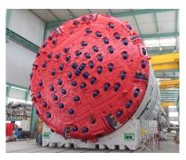
The Follo Line Project (Oslo, Norway): 40 km of Tunnels in Hard Rock Executed by 4 TBM Machines with Preliminary Grouting
