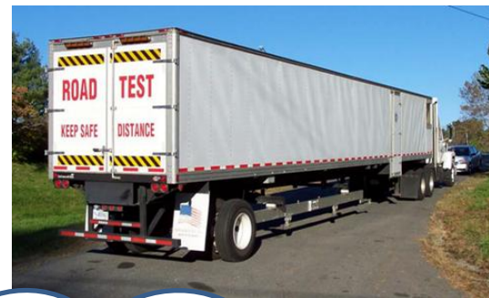
Rolling Wheel Deflectometer RWD
