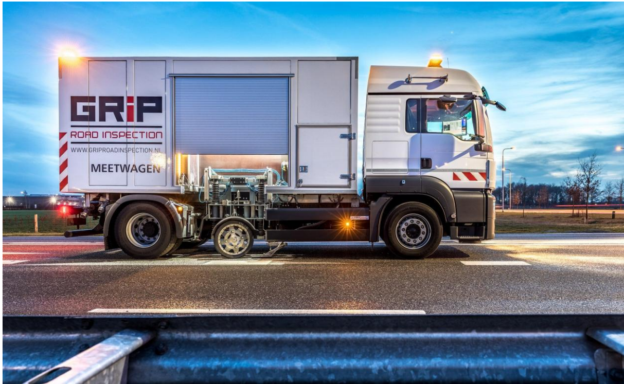
Figure 5: Sideway Force measure truck
